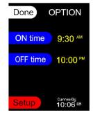
To RESTART the controller at any time, press the small green side button until you see the display briefly go blank. Restart SAVES your settings. **Try this first** if things don't seem to be working correctly or if you lose your place.
